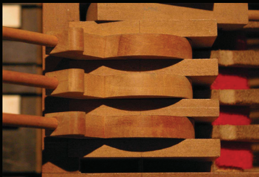
Hammer shanks and intermediate lever G. Silbermann piano
