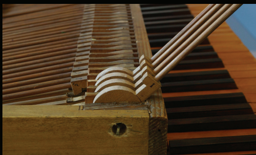
Hammer shanks and intermediate lever G. Silbermann piano
