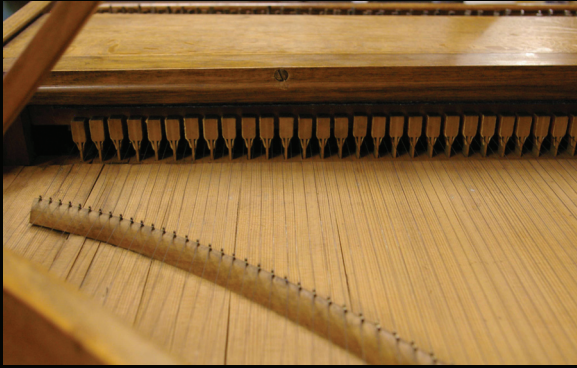
Equal spacing of strings in the pianos by Gottfried Silbermann
