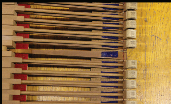
Hammer shanks and intermediate lever G. Silbermann piano
