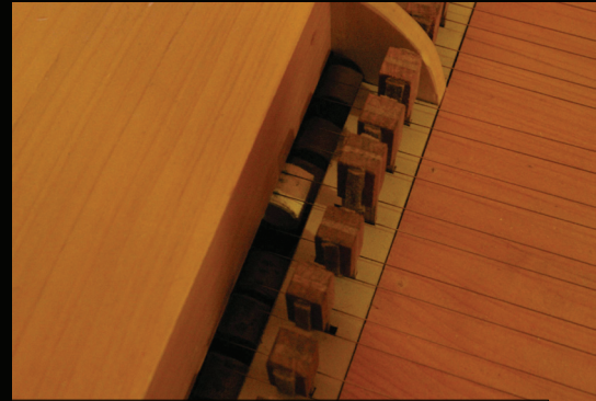
ill. 19, String spacing in pairs in Cristofori's pianos
