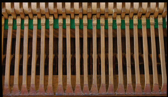
Hammer shanks and intermediate lever G. Silbermann piano
