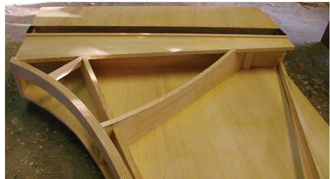
ill. 23, wide board glued behind the belly rail to prevent the registers being squeezed together
