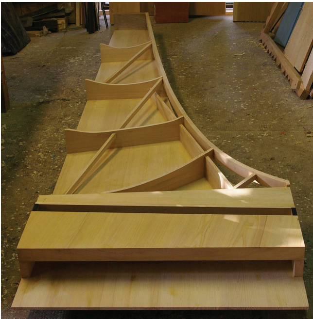
ill. 22, inner construction, copy of the ebony harpsichord
