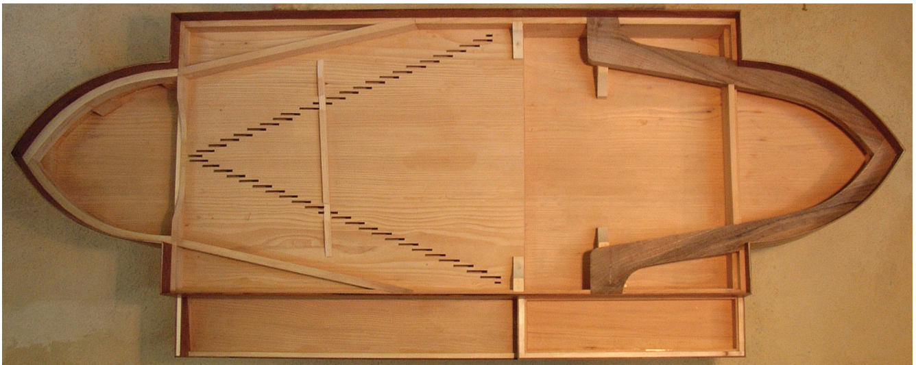
ill.13 the copy of the oval spinet, inner construction
